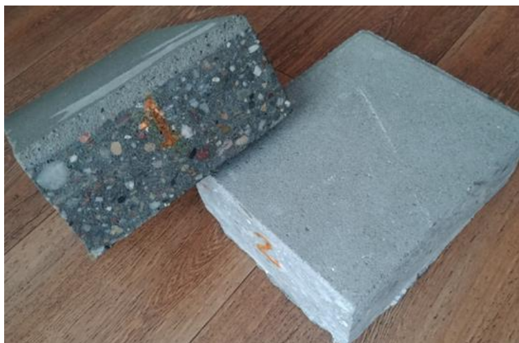
Fig. 1. Photocatalytic concrete paving block studied in the research. Figure from Witkowski et al. (2020).
