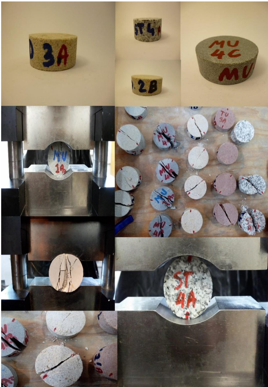
Fig. 9. Brazilian Test – laboratory experiment.
