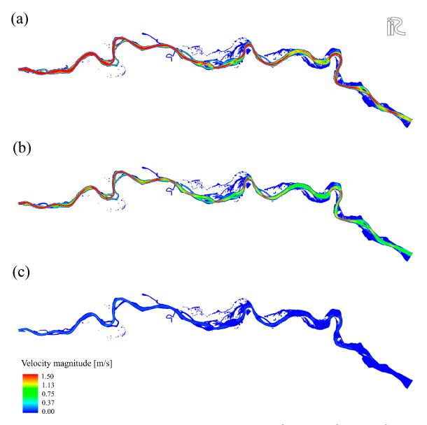
Figure 3. Simulated velocity profiles for the extreme events: (a) 5000 m<sup>3</sup>/s, (b) 3000 m<sup>3</sup>/s, (c) 200 m<sup>3</sup>/s.
