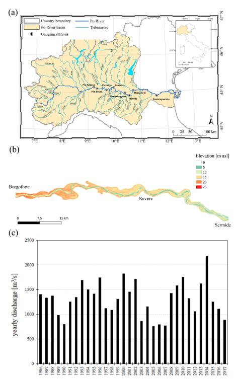
**Figure 1.** (a) Po River basin; (b) DEM of the studied area, from the upstream end of Borgoforte to the downstream end of Sermide; (c) yearly time series of flow discharge measured between 1986 and 2017 at the gauging station of Borgoforte (Mn).
